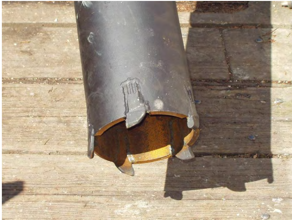
Figure 2-8 Serrated Edge of a Micropile
