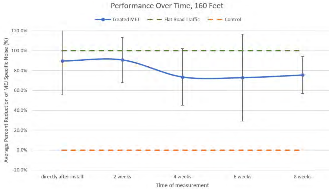
Figure 4-10. Comparison between untreated MEJ noise and the installed treatment over a two-month period at a distance of 160 feet.
